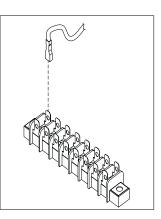
Figure 1-4 Plugging Quick Connects into the Terminal Block
